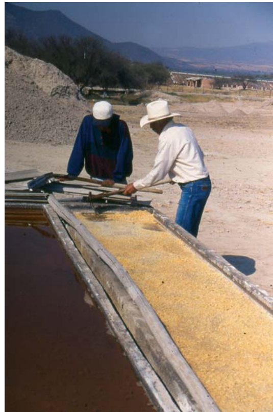
Salt Production in Mesoamerica. Fig. 3 The canoas are shallow troughs made with dugout pine trunks, used in the solar evaporation of brine. Note the crystallized salt on the right, the liquid brine on the left (© Eduardo Williams).
